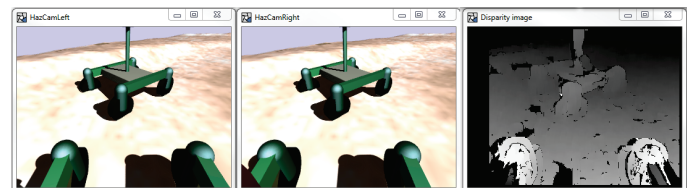
Figure 17: Left, right, and disparity images of a stereo camera.
